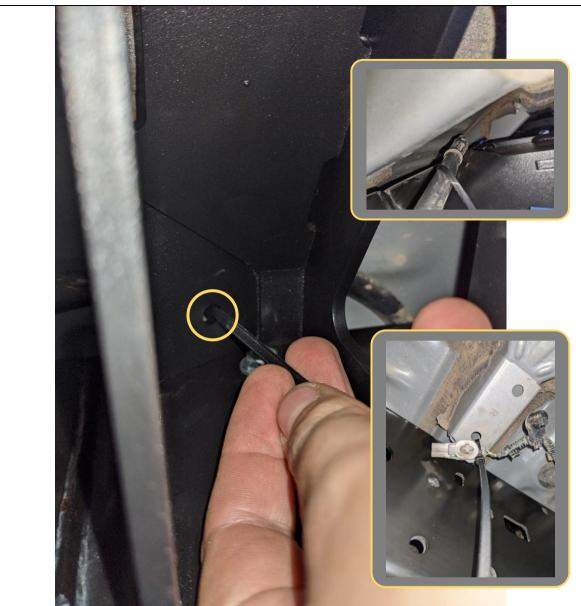
47. Secure Hand Brake cable and under step wiring harness with cable ties as shown in images.
