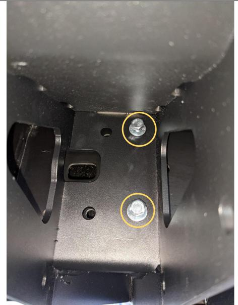
6. Fit the front mount, to the chassis using M8x20 bolts, HD flat washers, Secure finger tight only at this stage
