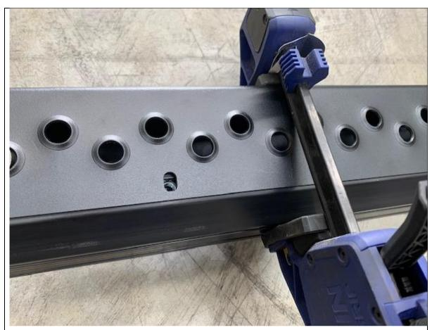
32. Using long tool feed nuts in to centre first and thread in with black M8 button head cap screws and washers.
