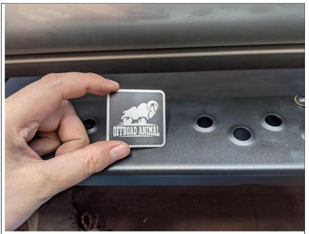
50. Fit the Offroad Animal logo plate to the small gap between pierced features on tread plate, using the pre applied double sided adhesive.
