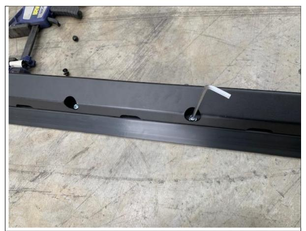
29. Thread cap screws into each hole.
